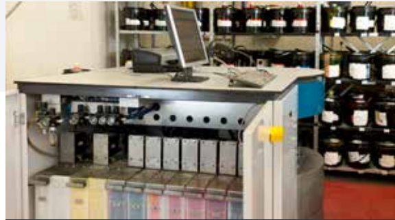
Internal storage tanks of the Colorsat Match
